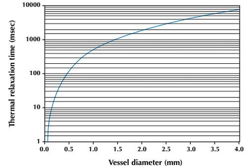
Figure 4—Thermal relaxation times for vessels ranging from 10 μm to 4 mm. ( $k=1.3 \times 10^3 \text{ cm}^2/\text{sec}$ ).
