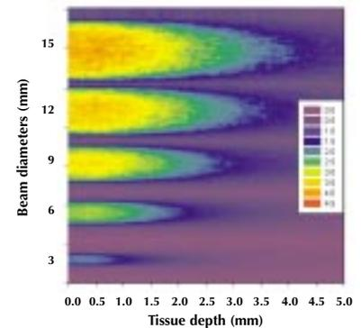
**Figure 2—Laser fluence distribution within dermis for 3, 6, 9, 12, and 15 mm beam diameters at 1064 nm.**
