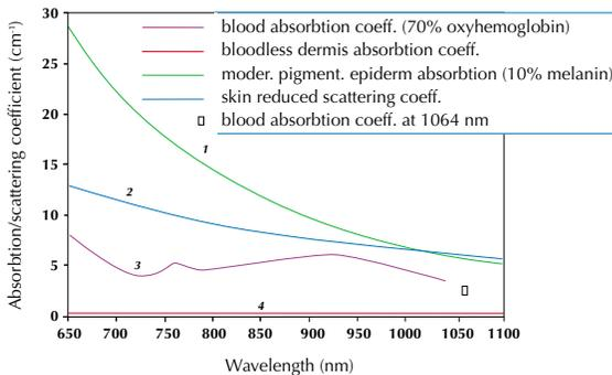
**Figure 1—Optical properties of blood, dermis and epidermis in the range of 650-1000 nm.**
