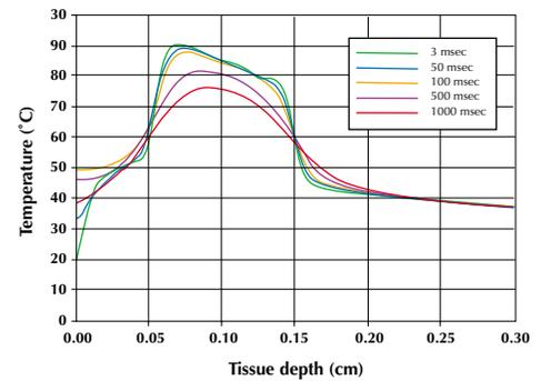
Figure 5—Temperature distribution inside a 1 mm diameter 1 mm depth vessel produced by 3, 50, 100, 500, and 1000 msec laser pulse durations.
